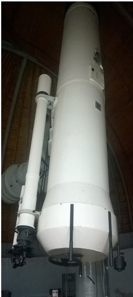
Figure 1: The Schmidt-camera 50/70 cm (NAO Rozhen, Bulgaria).
